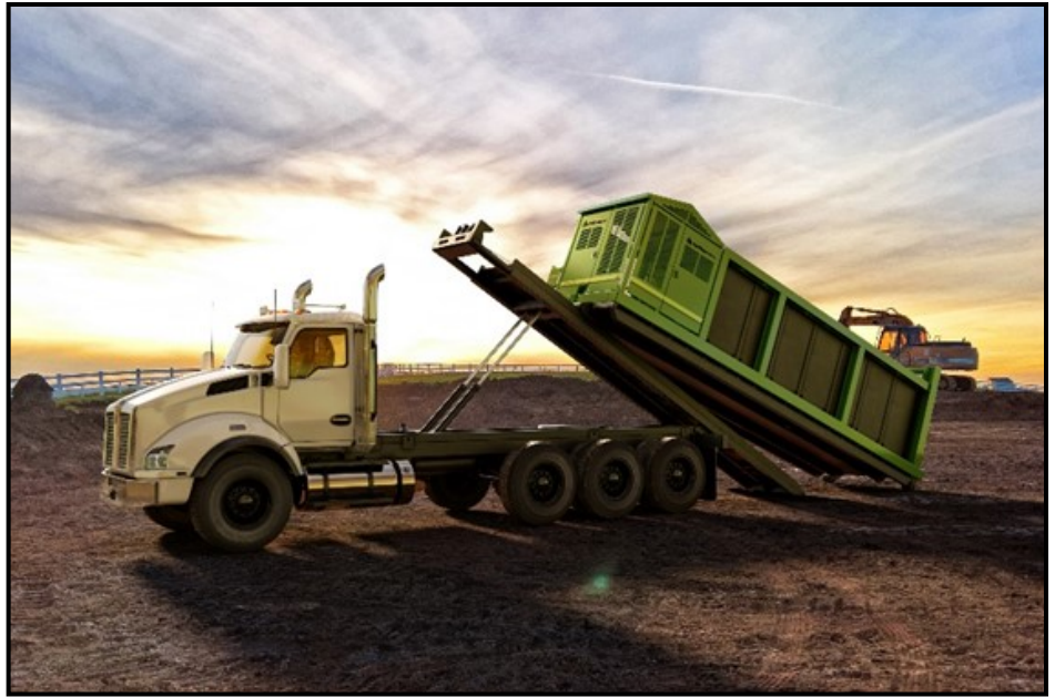
Roll-Off FireBox Being Delivered
