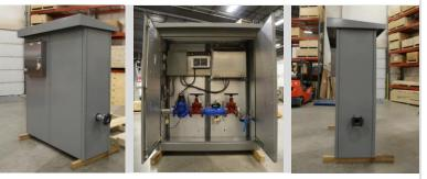
The FS-63 has all the features of the FS-43, including the ability to include multiple fill outlets and an attached solar panel, but is built with a larger painted steel enclosure to house additional piping such as strainers and pressure reducing valves.
