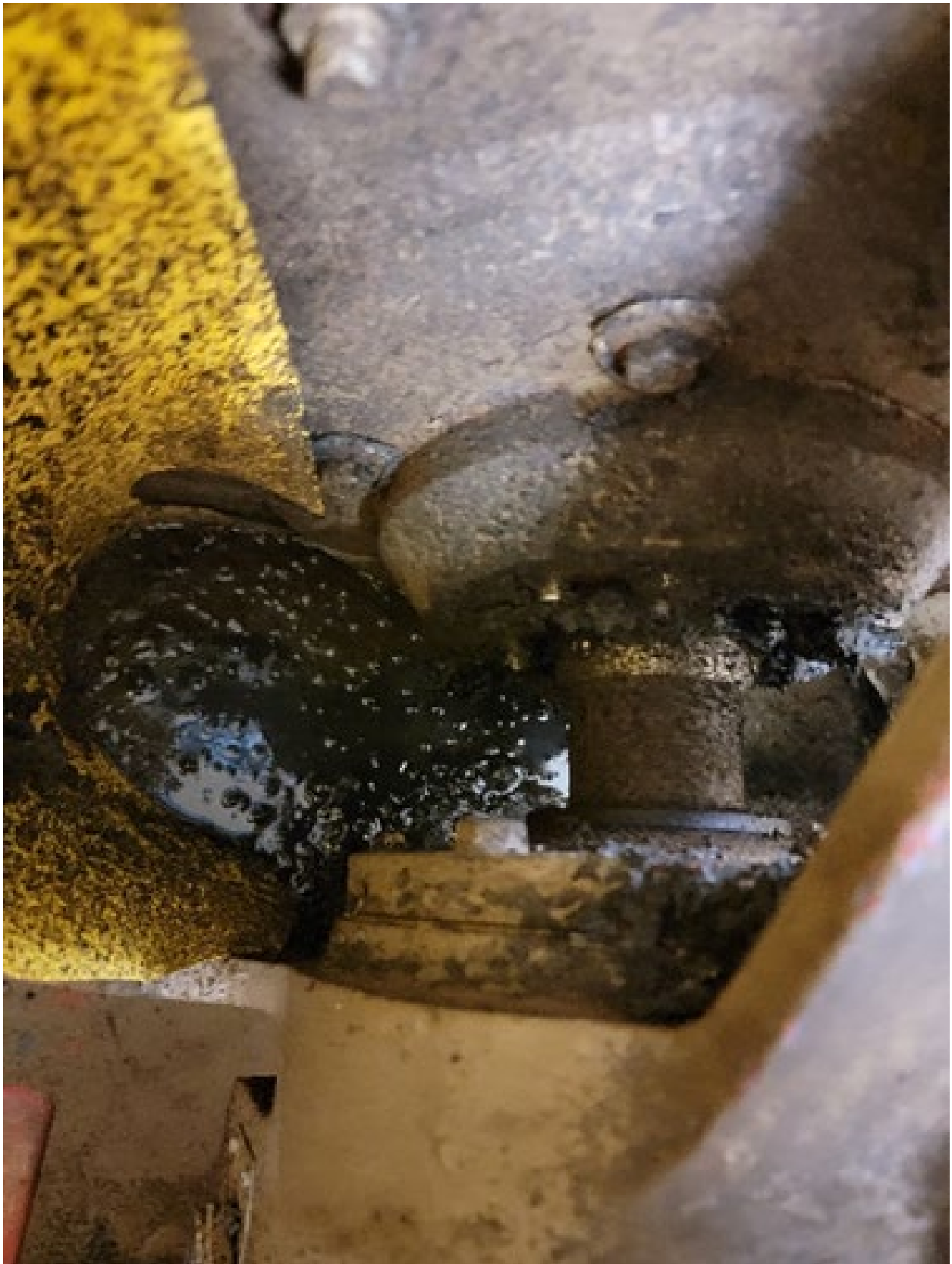
Figure 3: Bad Seal around Pump tied to Plugging Valve
