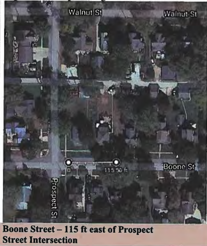
Figure 3: Example of Sight Distance Obstructed by Residential Structures
